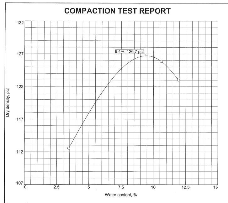
Test specification: ASTM D 1557-91 Procedure B Modified
