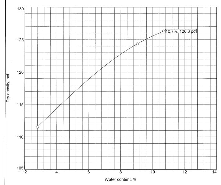
Test specification: ASTM D 1557-91 Procedure B Modified
