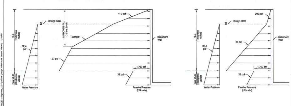
A. PASSIVE PRESSURE (ULTIMATE) UNDER SEISMIC CONDITION WITH IMPROVED FILL (UPPER 15 FEET)
